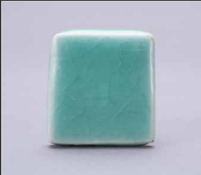
Fig. 4 Yongzheng test tile for imitation Longquan green glaze, inscribed “Changnei Longquan” (厂内龙泉, Longquan within factory) in cobalt, excavated from the Zhushan imperial kiln site, Jingdezhen. Collection of Tang Ying Society.
