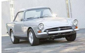
noted Tiger expert Paul Reisentz of Santa Clara, California's Reisentz Restorations rebuild the entire suspension and brakes during 2004-2005, with parts supplied by Sunbeam Specialties. The interior was refurbished at the same time. The suspension components were powder-coated, while Koni shock absorbers and a rear axle stabilizer bar provide sure-footed handling.
