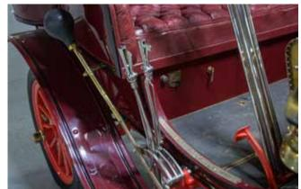
The Model Z represented something of a departure for the company as it had a plate clutch operated by pedal and sliding pinion gearbox, as opposed to the epicyclic system that they had used since the turn of the century, and a slightly larger motor. With these individual characteristics which were not repeated on subsequent models it makes identification of this rather rare model relatively straightforward.
