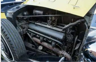
of 3AZ48. During Mrs. Fox's ownership, an engine knock was found to be incurable and the car was sent back to Rolls-Royce for service. On January 5th, 1938 it is recorded that the original engine, D54W, was removed and the "engine [was] taken out of 36EX & fitted into this chassis". As an early, experimental chassis, this unique, prototype motor that was never stamped but instead fitted simply with a plate reading "PHANTOM III UNIT NO. II" is the engine presently installed in the car.
