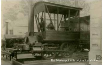
The Mississippi's service life spanned more than fifty years which in itself is remarkable for railway locomotive of the period. In the 1920s, then owner Illinois Central reported that the engine's weight was 19,700 lbs. (Not including the tender). An inspection in 1928 found that the locomotive was probably still capable of being steamed. Its present condition is largely the result of a substantial restoration in 1965 (see below).
