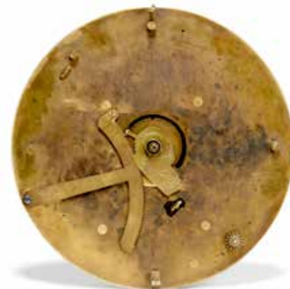
Equation cam removed to show the rack and pinion that varies the Solar hand. Additional views of the movement are available in the on-line catalog.
