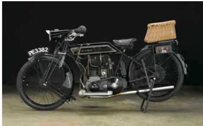
this tank is a piece of artwork to be appreciated like a Monet, Up front, a set of Druid forks cancel out the roughness of the roads with an acetylene lamp to light the way at night. This period British motorcycle used thumb levers to control the spark advance and throttle, unlike the twist grip throttles found on American motorcycles. The finish reflects the enjoyment of use and there is much original nickel plating on the motorcycle with original leather tool boxes.
