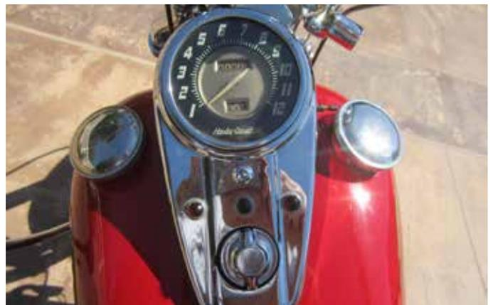
original zero miles Panhead speedometer that looks perfect on top of the tanks. Flanders risers and handlebars set atop the original, chromed forks. Other accessories include a cast aluminum spark plug holder, black solo leather seat, a Tombstone tail light and Cycle-Ray headlight wired to a 6 volt system.
