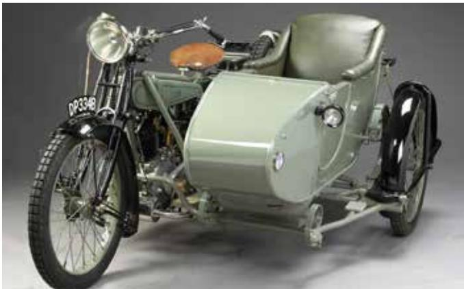
restored. The luggage platform at the rear with petrol can mounted underneath provide for the longer journey. The sidecar is believed to be of Clyno manufacture, coachbuilt to traditional standards and equipped with a detachable flexible windscreen. Interior fittings include a lockable cupboard and a separate toolbox.
