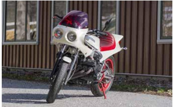
suspension and Brembo brakes. The tank, seat and fairing were specially customized, featuring twin head and twin taillights, and new 3-spoke, 17in wheels. The 6-into-1 exhaust system was handmade in stainless steel and the motor was modified to give 140 horsepower at the rear wheel but still maintain the original Honda drivability and reliability.
