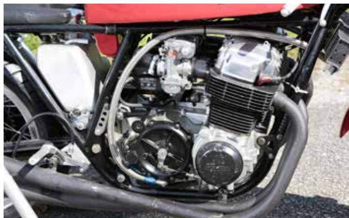
CB750F ('PVR 511R') purchased in April 2002. It is not known when it was last used. Noteworthy features include twin front disc brakes; 18" alloy wheel rims (Akront front, Morad rear); Avon racing tyres; an oil cooler; braided steel oil lines; Hagon shock absorbers; and Keihin CR carburetors. The machine comes with a substantial history file containing assorted correspondence, invoices and other paperwork (close inspection recommended).
