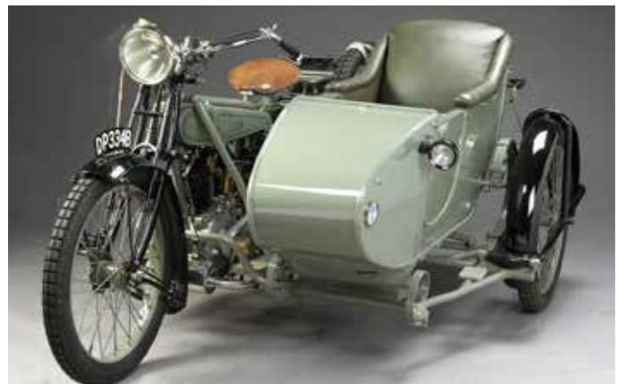
restored. The luggage platform at the rear with petrol can mounted underneath provide for the longer journey. The sidecar is believed to be of Clyno manufacture, coachbuilt to traditional standards and equipped with a detachable flexible windscreen. Interior fittings include a lockable cupboard and a separate toolbox.
