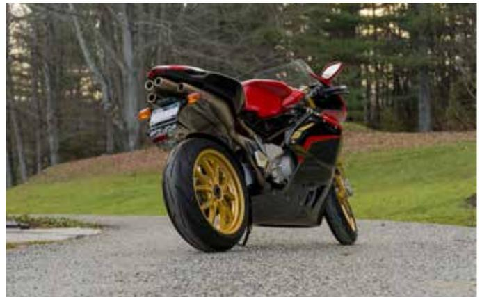
Only 300 limited edition Tamburini F4s were built for the world market. Each had a re-tuned 4-cylinder engine installed producing 173 horsepower, and included a magnesium swing arm and frame plates, a carbon fiber kit comprising air box, air ducts, tail fairing, front mudguard, side panels, and upper and lower chain guards, plus special graphics, an instrument panel with a stopwatch, and a gold serial number plate on the steering head.
