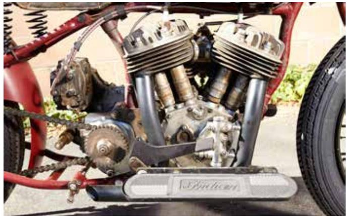
Today the reconstituted frame's main section and gas tank remain in their original, battle-worn paint, while the fork legs, rear frame section and fender have been repainted. Housed within the frame tubes – as it's been for the past 77 years – is the all-important factory Scout motor bearing its FCI-7 serial number and breathing through a Linkert carb set up to run on alcohol.
