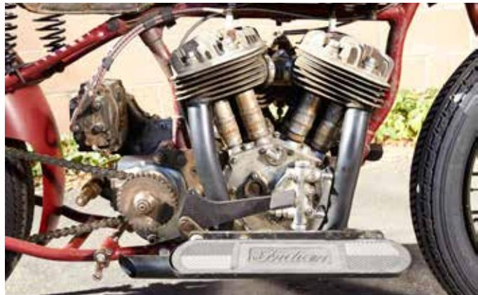
Today the reconstituted frame's main section and gas tank remain in their original, battle-worn paint, while the fork legs, rear frame section and fender have been repainted. Housed within the frame tubes – as it's been for the past 77 years – is the all-important factory Scout motor bearing its FCI-7 serial number and breathing though a Linkert carb set up to run on alcohol.
