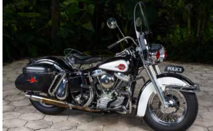
This 74 ci motorcycle is a basic FLH, meaning it has a hand shift, four speed transmission. There were three police option packages for 1960. FP-1 had the front fender mounted siren with hand control, speedometer hand control, oil filter and Deluxe solo saddle. FP-2 provided a foot control for the siren while the final option package FP-3 designated a rear mounted siren. With the sprung solo saddle, it was a comfortable ride.
