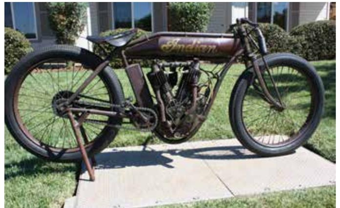
its as-raced condition. Amazingly, about 85% of the original parts remained. The engine was rebuilt to running condition, needing only a new set of pistons. A reproduction fuel tank, fork tubes, handlebars and rear stand were fashioned, carefully patina'd to match the frame's original faded red paint.
