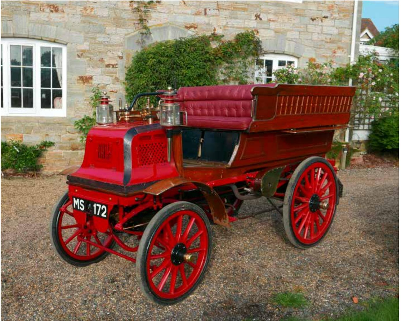
Built by the Daimler Motor Company of Coventry in 1897, this 4hp model has eight-seater Wagonette coachwork by Stirling of Hamilton, South Lanarkshire. Stirling's ordered substantial quantities of cars from Daimler, both complete and in chassis form; consequently, Daimlers were plentiful in Scotland before 1900. This particular model was produced from 1897 to 1900 and priced, when new, at £370.
