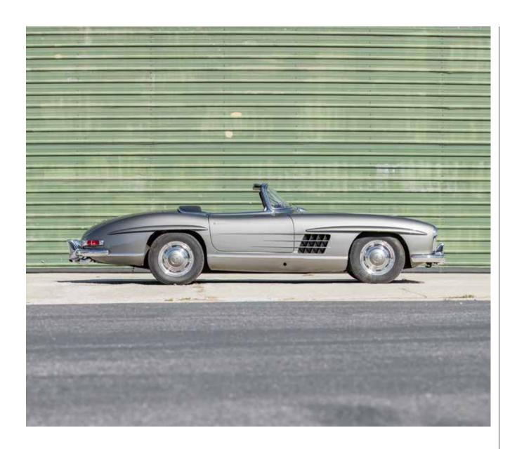
royalty, actors and socialites. The production of an open 300SL involved altering the cockpit area, where the spaceframe was redesigned to permit lower sills for improved access. At the same time the rear suspension was changed to incorporate low-pivot swing axles. The 300SL Roadster sold well for a car that cost more than a Ferrari 250 GT California Spider, and would out-live the 300SL Coupe by several years.
