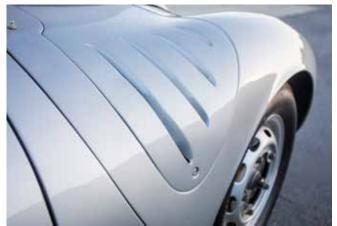
louvred hatches were also added in front of the rear haunches to maintain easy access to the motor for quick inspection. Additionally, the spare tire was stored up front for more ideal weight distribution. Smaller lighting treatments front and rear, again, make the 'a' model identifiable, while the subtlest change of all occurred up front with a reprofiled nose for better aerodynamics.
