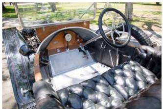
essentials: a Warner Auto-Meter speedometer/odometer and a sight glass oil indicator. The fuel tank and turtle deck are mounded to the frame immediately behind the body, with a single spare tire attached to the running board. The large windshield folds at the center, allowing for the top half to be folded down for ventilation even when the top is in place. The folding black fabric top is in very nice condition, and under the hood, the T-head four-cylinder engine is nicely detailed and presented.
