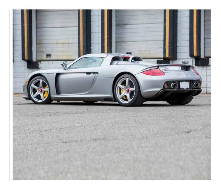
control arms all round with horizontally mounted gas shock absorbers operated via pushrods and rockers. Its brakes too are racetrack developed, consisting of six-piston aluminum calipers gripping 15" diameter ceramic composite discs that are more heat resistant and 50% lighter than castiron equivalents. More weight was saved from the wheels, which are made of forged magnesium (19" front, 20" rear) while ABS was standard equipment, as was power assistance for the steering.
