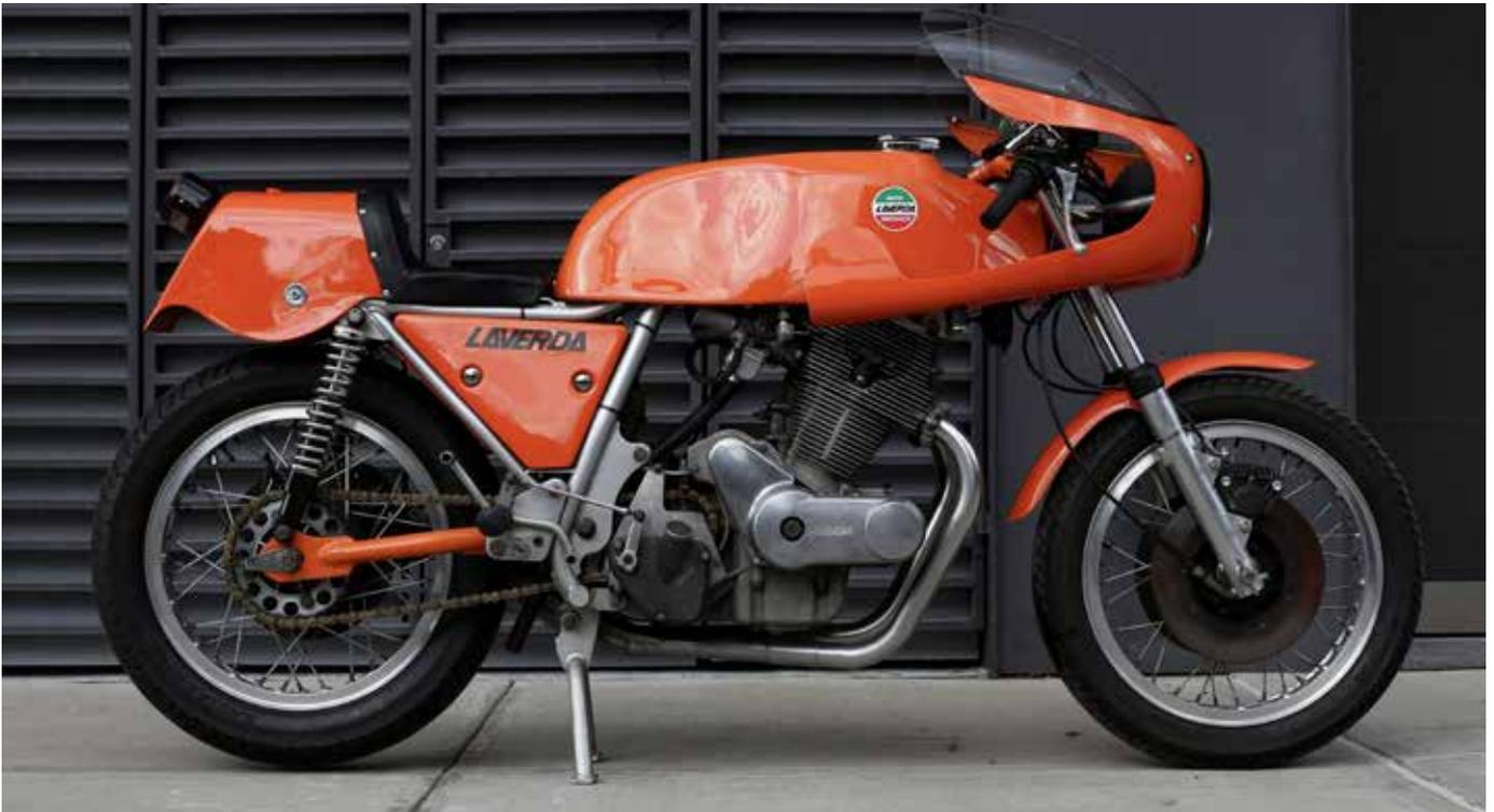
Two of the most significant updates for 1974 was the pair of Dell'Orto PHB 36 carburetors, without accelerator pumps, and twin-bleed Brembo F08 callipers with twin front discs, and a single rear disc on an Elektron hub. A racing two-into-one megaphone (as on this example) accentuated the lean race replica profile, and the claimed power for the 1974 750 SFC was 75 horsepower at 7,500 rpm. The right-side gear shift remained as did Borrani rims and Ceriani suspension front and back.
