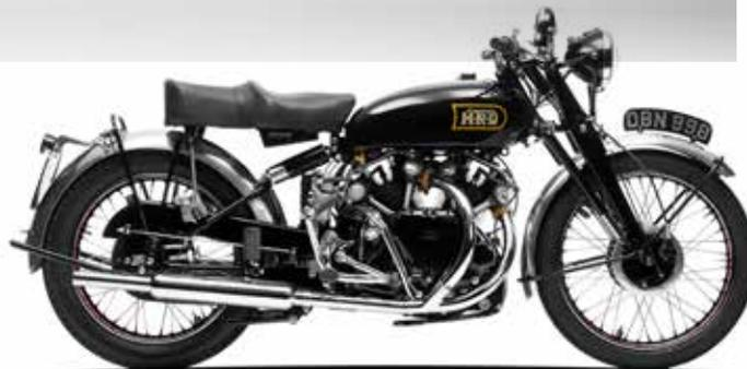
The most significant changes made concerned the suspension, there being a revised arrangement at the rear incorporating curved lugs for the seat stays and an hydraulic damper between the spring boxes, while at the front the new models boasted Vincent's own 'Girdraulic' fork: a blade-type girder fitted with twin hydraulic dampers.
