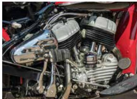
In 1937, Harley Davidson introduced a new series model called W that featured a 45 cubic inch engine and more importantly a recirculating oil system that was supposed to reduce maintenance and increase reliability. This was specifically convenient for the rider that did not need to check the oil, adjust the oil pump or even lubricate the engine while riding anymore. Harley quickly received an order from the US Army to replace its fleet of RL models.
