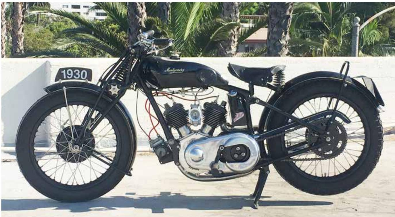
This J.A.P. engine is a sidevalve motor of 750cc displacement with air-cooled covers over the exhaust valves. The highly polished engine cases are a delight to enjoy. Ignition is provided by magneto located forward of the engine. An Albion gearbox with a 3-speed hand shift completes the package. It can be described as a touring motorcycle capable of extended use at a high rate of speed. Unfortunately, World War II forced the small English company to shut down and production ceased in 1939.
